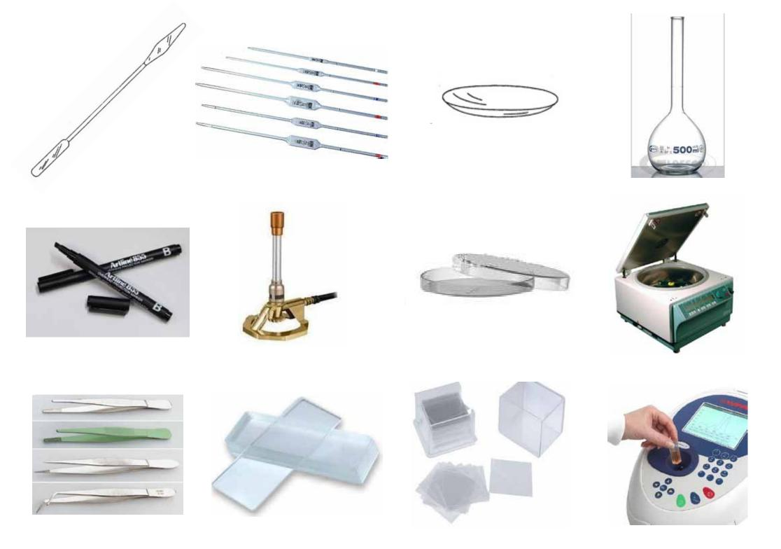
A spatula is used to transfer solids. It is often used to transfer solids from a container into a weighing vessel. Avolumetric pipet measures and delivers exact volumes of liquids and has a single graduation that allows it to deliver one specific volume accurately.
