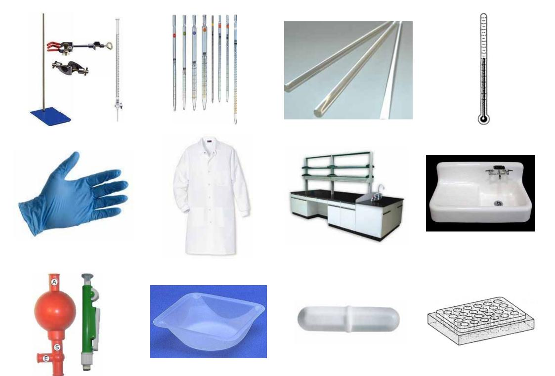
Burets are usually made of glass and contain many markings, called graduations. Burets are used to measure and dispense liquid volumes accurately. It is used with a ring stand as a support and
